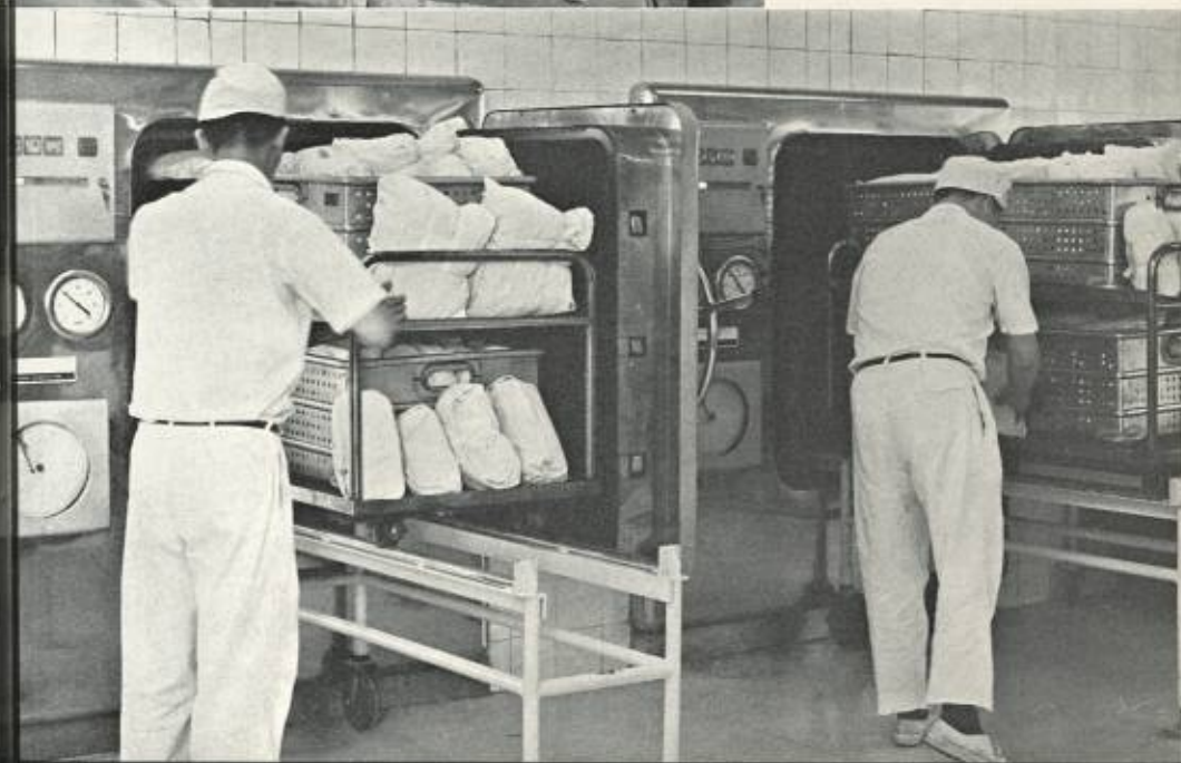
Central Sterile Supply Department, Queen Elizabeth Hospital —Packed instruments being delivered to the autoclave for sterilization.
